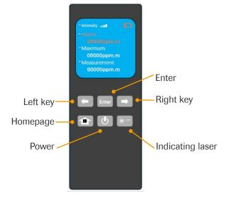
**Power:** In the shutdown state, long press (5s) to turn on the device; When turned on, long press (5s) to turn off.
