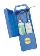
Through our on-going improvement programs, the use of the genie ozone generator was reviewed, and we have also been using the ATi ozone generator. The ATi utilizes a UV-Light process which converts some of the oxygen from a 'dry air' cylinder to ozone.
