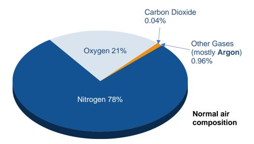
Obtaining calibration gas with Methane in a true air background is not always possible. In order to make sensor testing on-site as simple as possible, the sensor algorithm has been adapted to produce a correct Methane response when a mixture of 2.2% Methane and 18% oxygen in a background of nitrogen is applied. The lower concentration of oxygen in the test gas offsets the sensor response in proportion to the absence of Argon, resulting in an accurate calibration.
