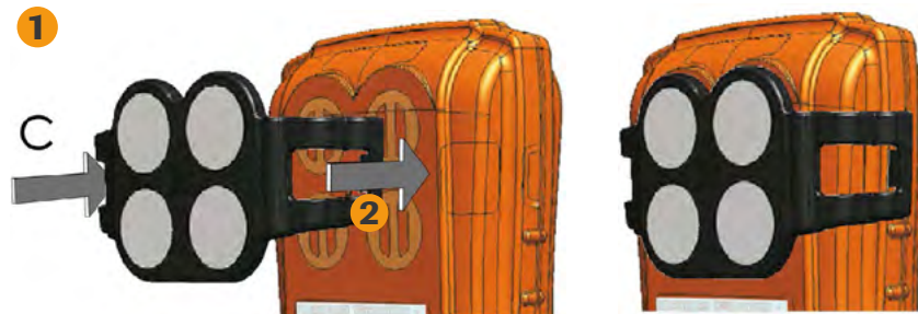
Figure 6: Installation de la plaque de filtres externe
