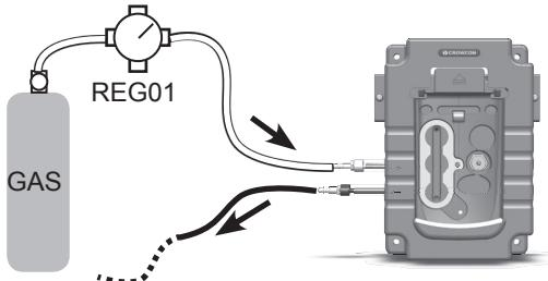
NB. The fixed flow regulator should be switched on at all times to maintain a pressure up to 3bar.
