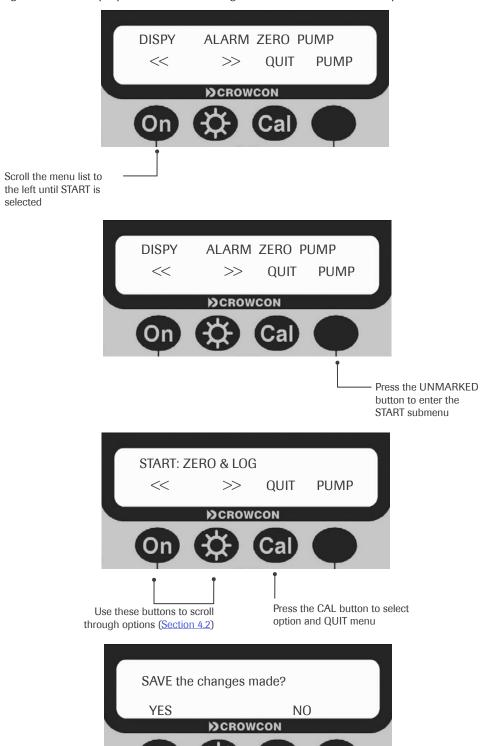
Press the first button to save the change and move the menu back up a level, and the last key to leave the selection as it was (unchanged) and move back up a level.
