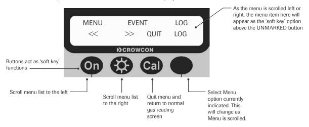
The four buttons have above them a symbol or word: these are the 'soft key' functions currently assigned to that particular key. Use the ON and BACKLIGHT buttons to scroll left and right, the CAL button to quit the menu system and the UNMARKED button to select a menu option. View the road map on page 37 for details of **Detective+** configuration menu system
