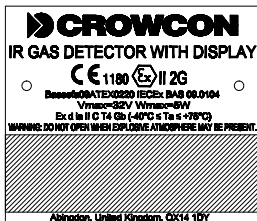
Diagram 1 Certification label fitted to IRmax compatible with the IR Display
